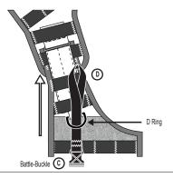
Loop Battle-Buckle "C" back through the loop end "D" of the HARNESS STRAP. Tighten the loop until it is snug against the D Ring.
