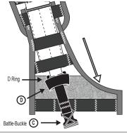
Connect Battle-Buckle "C" of the HARNESS STRAP to Battle-Buckle "B" of the WEAPON MOUTING STRAP.
