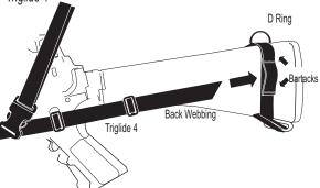
Place your fist between the sling and the rifle, as shown, and insert the Front Webbing through the M-16 Front Attachment Point
