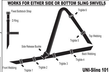
Insert the loose end of the Fixed Buttstock Strap through the triglide and secure it Triglide Fixed Buttstock Strap
