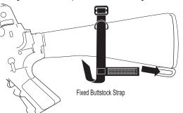
Insert the Back Webbing of the UNI-Sling 101 through the loop created between the Bartacks on the Fixed Buttstock Strap and secure it using Triglide 4
