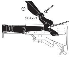
Connect Battle-Buckle "C" of the FRONT TRAVERSING STRAP to Battle-Buckle "G" of the SHOULDER STRAP. Use the "Speed Adjuster", Slip lock 2 and 3 for adjustment purposes.
