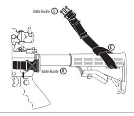
Connect Battle-Buckle "B" of the FRONT TRAVERSING STRAP to Battle-Buckle "D" of the REAR TRAVERSING STRAP.
