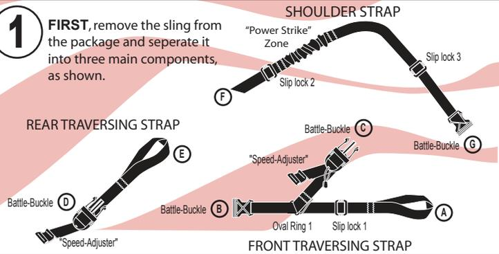
**2** Pass the loop end "A" of the FRONT TRAVERSING STRAP through the front sling mount of the weapon. Then feed Battle-Buckle "B" back through the loop end "A" followed by the rest of the FRONT TRAVERSING STRAP.
