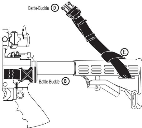
**5** Connect Battle-Buckle "B" of the FRONT TRAVERSING STRAP to Battle-Buckle "D" of the REAR TRAVERSING STRAP.
