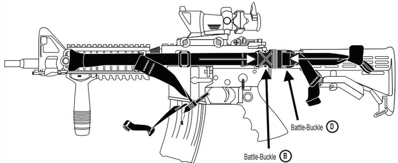
**6** Pass end "F" of the SHOULDER STRAP through the loop created by the REAR TRAVERSING STRAP as shown and then thread end "F" through Slip lock 2.
