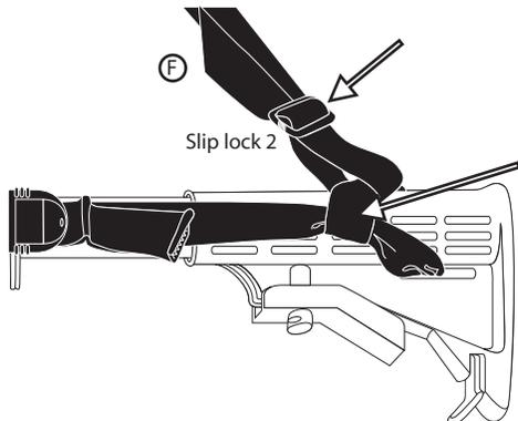
**7** Connect Battle-Buckle "C" of the FRONT TRAVERSING STRAP to Battle-Buckle "G" of the SHOULDER STRAP. Use the "Speed Adjuster", Slip lock 2 and 3 for adjustment purposes.
