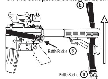
**4** Pass Battle-Buckle "D" of the REAR TRAVERSING STRAP through the loop end "E" as shown.
